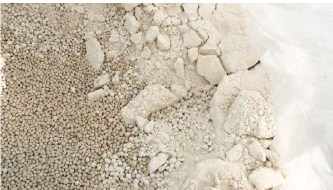
Avoid storing bagged AN-based fertilizers outdoors during the summer season; risk of thermal cycling leading to dust formation.
