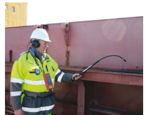
Testing for leaks by ULD
