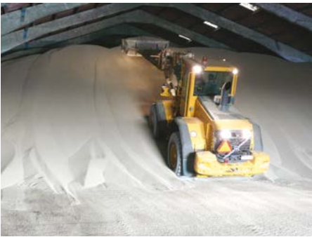
UNACCEPTABLE driving into pile
