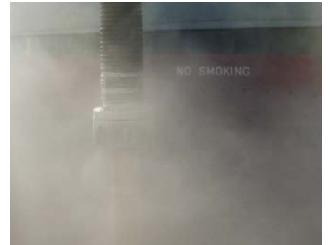
Excessive dust during loading vessel
