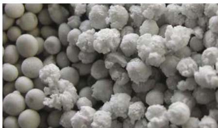
Disintegrated fertilizer due to water absorption
