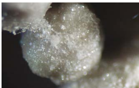
Crystal bridges between fertilizer particles cause caking
