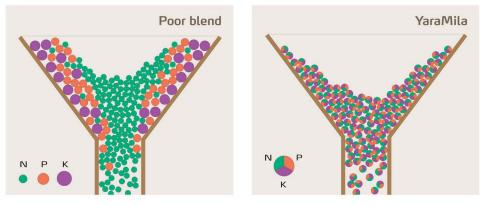
Segregation can cause poor spreading patterns, which lead to financial losses. YaraMila's hard prill, improves spreading and reduces waste. (Trials have shown that a 30% variation in spreading patterns due to segregation of poor quality blends can affect the bottom line for, for instance, winter wheat by more than 18 USD/ha!)
